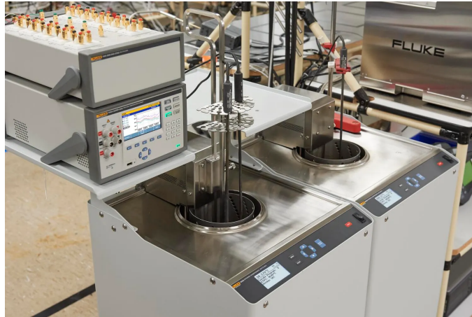
Comparison calibration of temperature sensors and instruments against traceable reference standards
