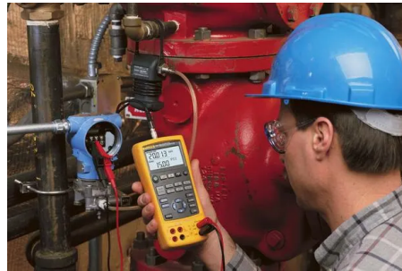
Field verification confirms instrument accuracy against traceable reference standards
