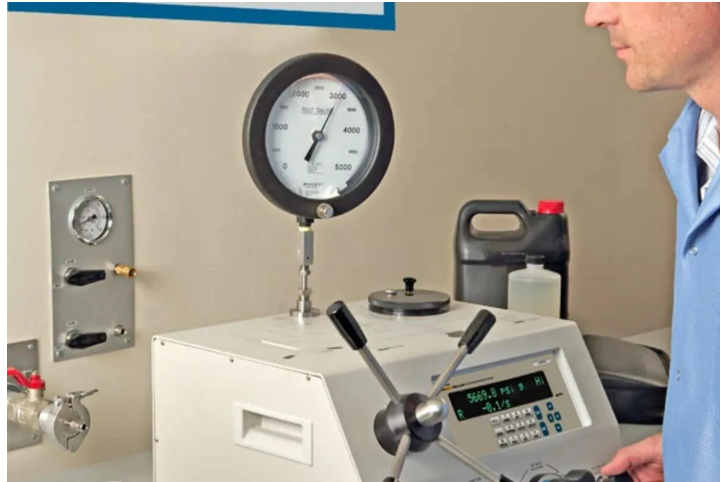
Comparison calibration of pressure gauges, transmitters and switches against traceable reference standards
