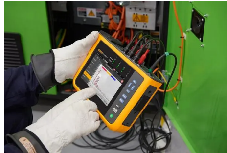
Field measurement of power-quality parameters to IEC 61000 and IEEE 519
