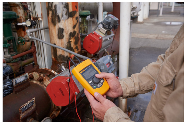
As part of custody transfer, technicians routinely calibrate all the pressure and temperature transmitters involved in the flow of oil & gas
