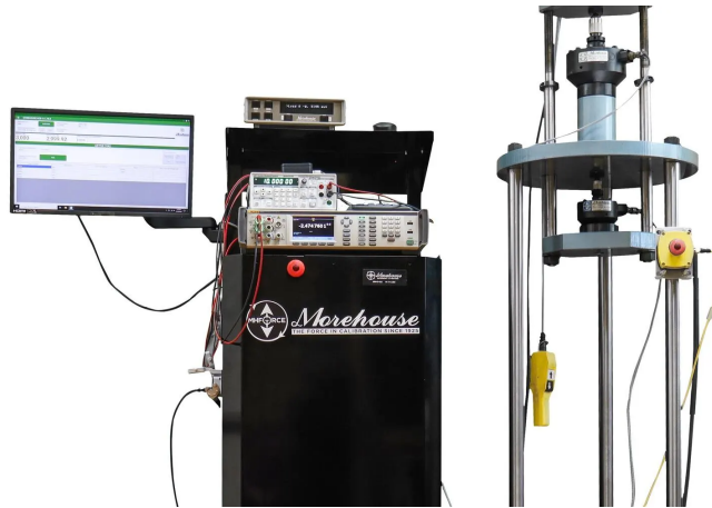
Comparison calibration of mass and force instruments against traceable reference standards
