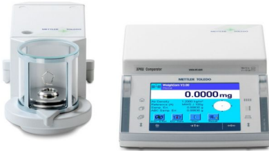
A precision mass comparator calibrates weights against reference standards
